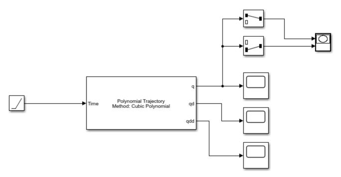
Run the simulation. The first figure shows the output of the q vector for the positions of the trajectory. Notice the cubic polynomial shape to the trajectory between waypoints. The **XY Plot** shows the actual 2-D trajectory, which hits the waypoints specified in the block mask.
