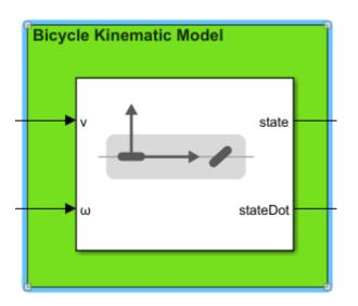
Bicycle Kinematic Model creates a vehicle model to simulate simplified vehicle dynamics. It takes linear and angular velocities as input from the Pure Pursuit Controller block, and outputs i.e. state and stateDot which are the robot's state and the robot's state's time derivative, respectively. The robot' state is also used to calculate the the distance to goal and check if the robot has reached the goal location.
