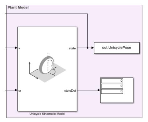
The **Unicycle Kinematic Model** block creates a vehicle model to simulate simplified vehicle kinematics. The block takes linear and angular velocities as command inputs from the **Pure Pursuit** controller block, and outputs the current position and velocity states.
