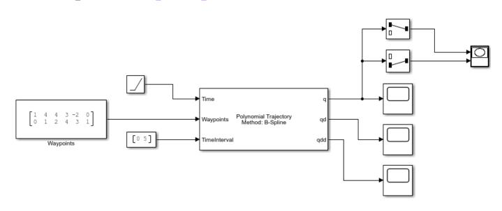
Run the simulation. The first figure shows the output of the **q** vector for the positions of the trajectory. The **X Y Plot** shows the actual 2-D trajectory, which stays inside the defined control points and hits the first and last waypoints.
