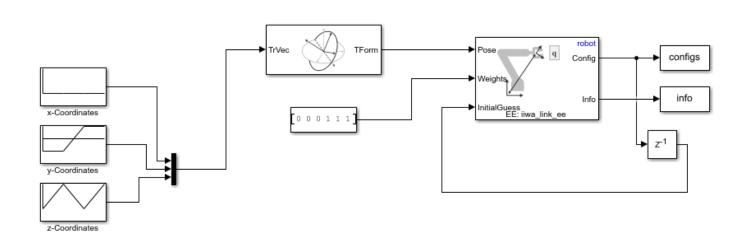
% Run the simulation. The model should generate the robot configurations (configs) that follow the specified trajectory for the end effector.
