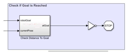
If robot has reached the goal location, the simulaion is stopped.
