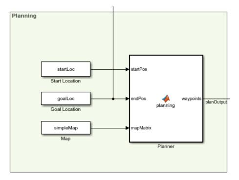
The **Planner** MATLAB® function block uses the mobileRobotPRM path planner and takes a start location, goal location, and map as inputs. The blocks outputs an array of wapoints that the robot follows. The planned waypoints are used downstream by the **Pure Pursuit** controller block.
