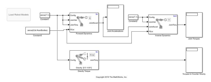
The Forward Dynamics block calculates the joint accelerations due to gravity for a given lbr robot configuration with no initial velocity, torque, or external force. The Inverse Dynamics block then computes the torques needed for the joint to create those same accelerations with no gravity by using the lbr2 robot. Finally, the Gravity Torque block calculates the torque required to counteract gravity for the lbr robot.
