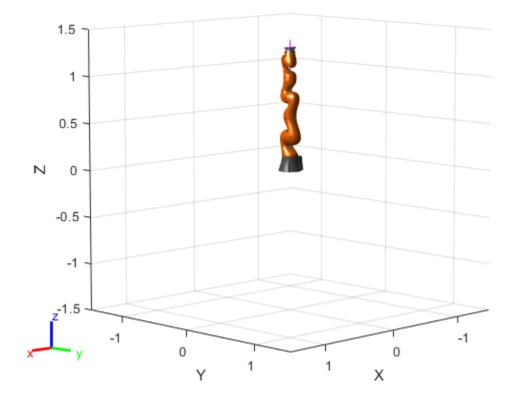
Open the model. The **Transform Trajectory** block interpolates between the initial and final transformation specified in the block mask. These transformations are fed to the **Inverse Kinematics** block to solve for the robot configuration that makes the end effector reach the desired transformation. The configurations are output to the workspace as configurations.
