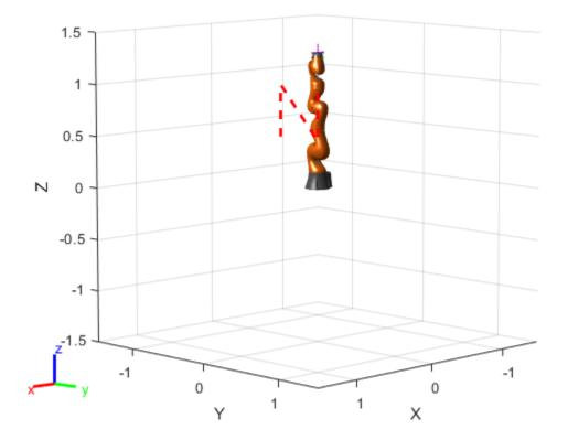
Open a model that performs inverse kinematics. The *xyz*-coordinates defined in MATLAB® are converted to homogeneous transformations and input as the desired **Pose**. The output inverse-kinematic solution is fed back as the initial guess for the next solution. This initial guess helps track the end-effector pose and generate smooth configurations.
