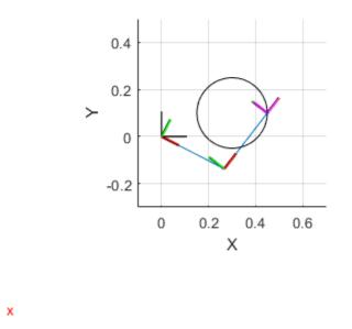
Set up a rateControl object to display the robot trajectory at a fixed rate of 15 frames per second. Show the robot in each configuration from the inverse kinematic solver. Watch as the arm traces the circular trajectory shown.
