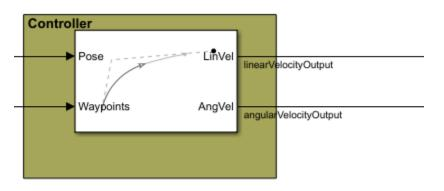
Controller outputs the linear velocity and angular velocity based on the waypoints and the robot's current pose. The Pure Pursuit Controller block is used for the same.
