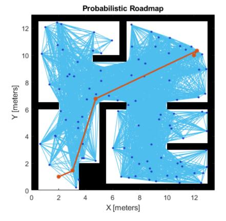
Reload the random number generation settings to have PRM use the same nodes. Lower ConnectionDistance to 2 m. Show the calculated path.
