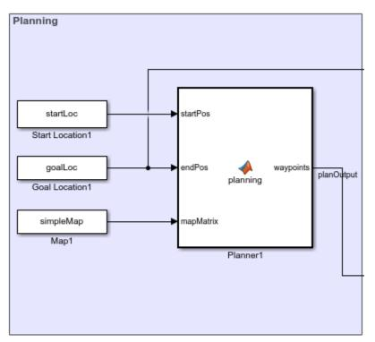
The **Planner** MATLAB® function block uses the mobileRobotPRM path planner and takes a start location, goal location, and map as inputs. The blocks outputs an array of waypoints that the robot follows. The planned waypoints are used downstream by the **Pure Pursuit** controller block.
