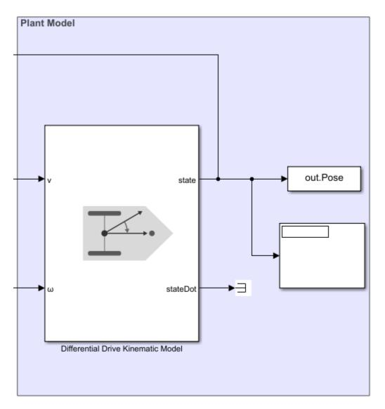
The **Differential Drive Kinematic Model** block creates a vehicle model to simulate simplified vehicle kinematics. The block takes linear and angular velocities as command inputs from the **Pure Pursuit** controller block, and outputs the current position and velocity states.
