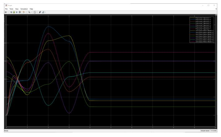
Observe that the signals for the first joint start separated, and overlap when time is equal to 1s. So from the initial configuration, the first joint was able to follow the trajectory.
