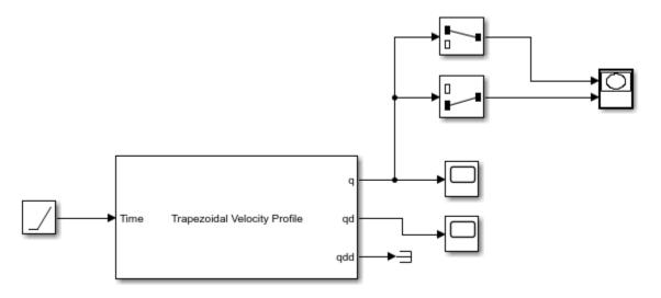
Run the Simulation. The first figure shows the output of the q vector for the positions of the trajectory. The second figure shows the qdd vector for the velocity. Notice the trapezoidal profile for each waypoint transition. The **XY Plot** shows the actual 2-D trajectory, which hits the specified waypoints.
