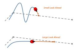
The LookAheadDistance property should be tuned for your application and robot system. Different linear and angular velocities will affect this response as well and should be considered for the path following controller.
