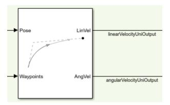
The **Pure Pursuit** controller block generates the linear velocity and angular velocity commands based on the waypoints and the current pose of the robot.
