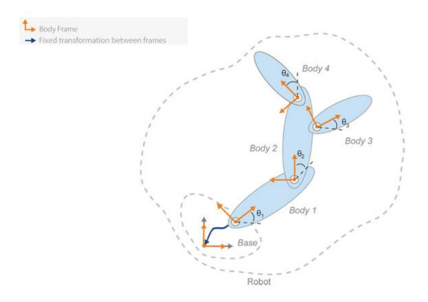
Use robot configurations when you want to plot a robot in a figure using **show**. Also, you can get the transformation between two body frames with a specific configuration using **getTransform**.
