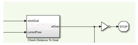
The **Check Distance to Goal** subsystem calculates the current distance to the goal and if it is within a threshold, the simulation stops.
