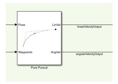
The **Pure Pursuit** controller block generates the linear velocity and angular velocity commands based on the waypoints and the current pose of the robot.
