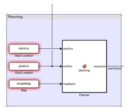
This blocks takes a start location, a goal location and map as inputs and outputs an array of wapoints which robot will follow. The planned waypoints are used downstream by the Pure pursuit controller which outputs the angular and linear velocities given the current pose of the robot and the planned waypoints as inputs.
