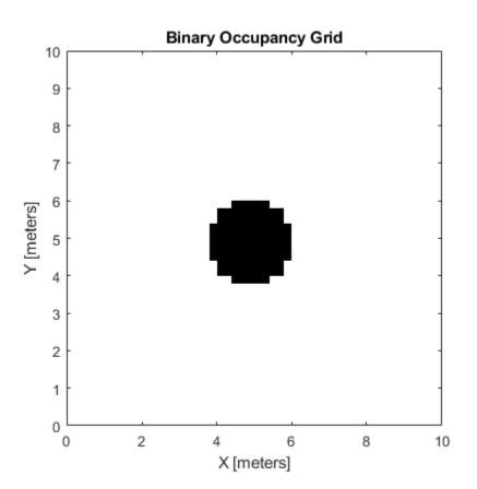
Plot original location, converted grid position and draw the original circle. You can see from this plot, that the grid center is [4.9 4.9], which is shifted from the [5 5] location. A 1m circle is drawn from there and notice that any cells that touch this circle are marked as occupied. The figure is zoomed in to the relevant area.
